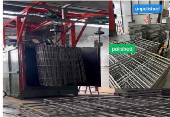
Derusting machine remove the rust and polish frame
